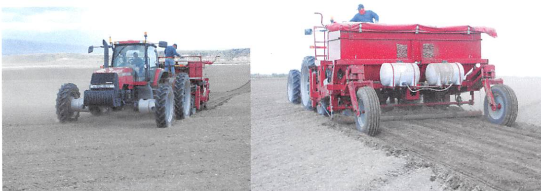
Figure 10. Planting with the Spudnik bedded planter. The ground is prepared as normal but no pre-marker is necessary. After ground preparation, the bed planter is ready.
