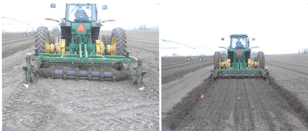
Figure 11. The modified Dammer Diker for a bed system. The outside paddles are 'normal', the inside paddles are used for a 'smaller' insertion into soil.
